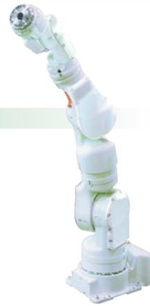
Note. High degree of motion like a human arm with its 7-axis arm.
