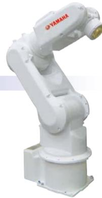
Note. The YA-R3F, a compact manipulator with a motor of 80 W or less mounted on all axes, requires minimal space (baseplate: 240 mm × 170 mm). No fence is required for robot's working area. The robot can be used in applications such as automated guided vehicles (AGVs), testing equipment, and educational tools.
