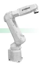
Note. Thanks to the higher control rate of the YAC100 controller and vibration-damping control of the arm, we have reduced the residual vibration when the arm stops moving, while shortening the cycle time and achieving the fastest speed in this class. Note. Longest reach in a respective class (895 mm)
