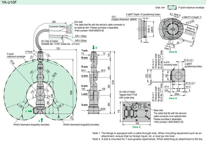
Note 2. A bolt is mounted for T-axis grease replenished. When attaching an attachment to 80 dia. -0.035/0 part of the T-axis, enough space for the grease zerk (A-MT6X1) is required to the shape of the attachment.
