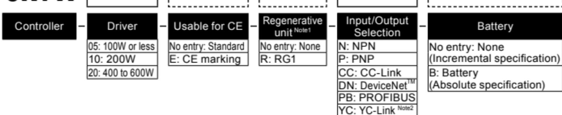
Note 1. Driver selection and regenerative unit selection depends on the robot type. See the selection table on the next page for selecting the driver/regenerative circuit.
