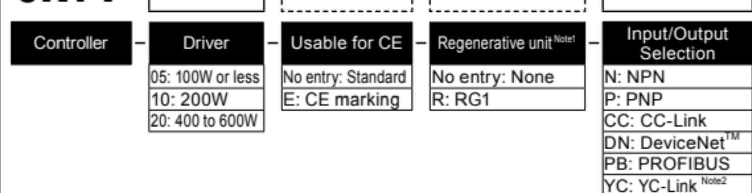
Note 1. Driver selection and regenerative unit selection depends on the robot type. See the selection table on the next page for selecting the driver/regenerative circuit.
