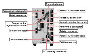
Note. Photograph shows RCX222. The component names on the RCX221 are the same but it does not come with an absolute backup battery.
