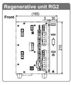
Note. Depth (D) is 158mm. Installs on the right side of the RCX221 (HP), RCX222 (HP). Cannot be installed as a separate unit.
